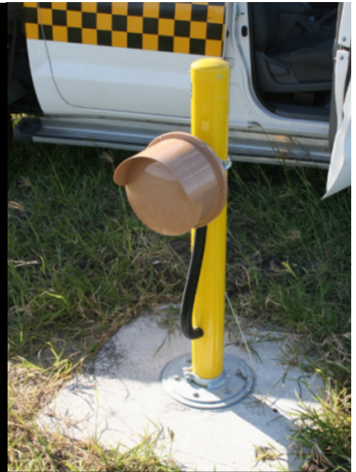
Southwest Microwave Volumetric Stop Bar Control Sensors at Sydney Airport. Source: Sydney Airport
